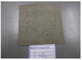
Fig 2. Water hyacinth bio-board successfully produce
